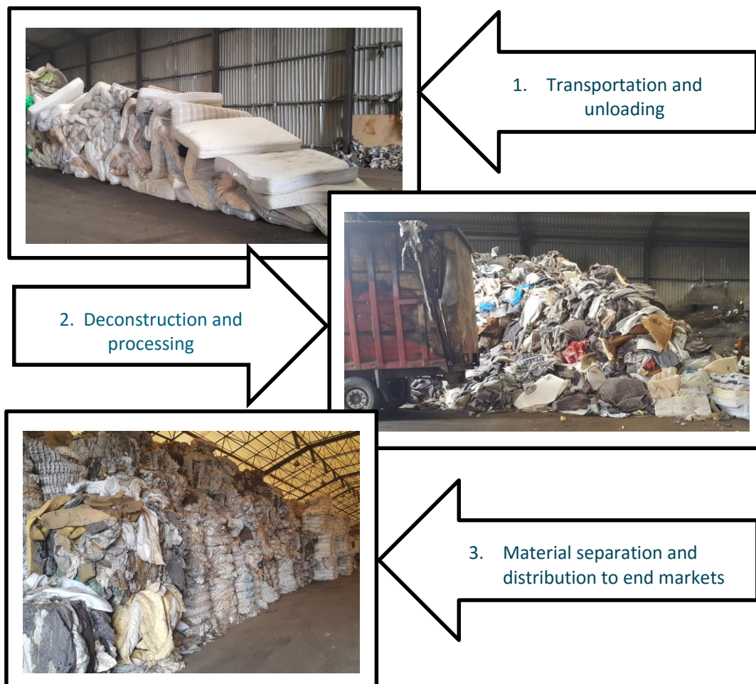
Figure 25: Diagram of typical mattress recycling process flow
